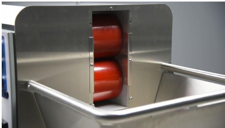
3. Remove the rear Lexan window to expose the chipper assembly.
