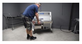
With the window and fascia correctly installed, let's slide the separator into place. There's a rail on the left side of the separator that carries the weight on the left side, but there is nothing carrying the weight on the right side.
