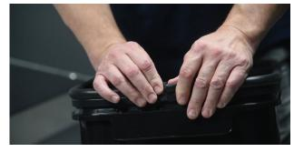
There shouldn't be anymore than  $^{1}/_{4}$ " of gap where the two ends of the gasket meet.
