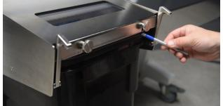
When you pull the latches up into place there should be no gap between the trim tote gasket and the underside of the separator. 12
