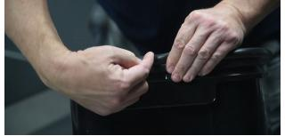
The trim tote gasket should b utt together above the warning logo on the trim tote. This gasket is an integral part of the vacuum system and should completely seal the top of the trim tote.
