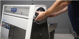
If you're using an infeed conveyor, be sure to install the infeed conveyor guide. This will all you to roll in the infeed conveyor into place.
