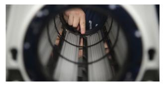
Be sure to perform a 6-point inspection. Make sure the clearance between the tumbler wires and the bed knives are the same at all 6 points.
