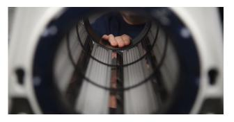
Give the tumbler a spin by hand in both directions to double-check that the tumbler wires aren't hanging up on anything.
