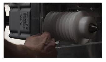
To reinstall a belt, start by working it onto each of the four rollers, aligning it into the same channel on each roller.
