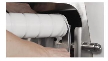
To re-install the rollers and belts, simply reverse the process. Start with the belt tension assembly set to the highest position so that you have maximum slack to work with.
