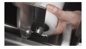
Both rollers on the outfeed side and the top roller on the infeed side can be removed by simply lifting them out of their cradling brackets.
