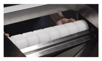
Removing the rollers can be done with or without the belts in place. So long as there is no tension on the belts, it is easy to work around them.
