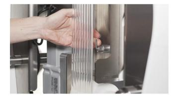
Locate the belt tensioner on the infeed side of the M9, pull out the adjustment plunger.
