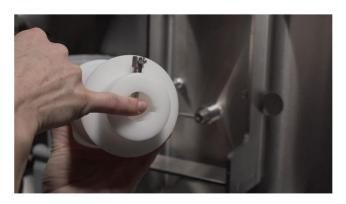
The bottom, or drive, roller on the infeed side is secured in place with a locating pin. Pull up on the pin to release the roller and pull it out of its cradling bracket.
