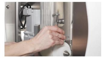
Move the entire assembly up to the maximum height, which will take the tension off the belts.
