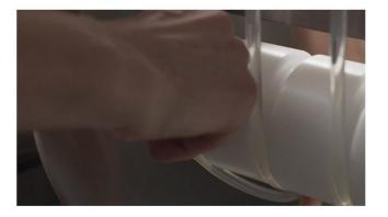
Working through the openings on the two ends and the tailgate, pull a belt away from the four rollers and out of the machine.
