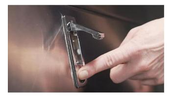
Move to the back side of the Sorter and open the tailgate by releasing the two compression latches.
