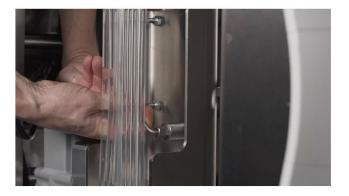
Once all of the rollers and belts are in place, pull the adjustment plunger and lower the tension assembly to the desired position.
