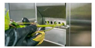
Begin feeding the bottom end of your stalks into the holes in the die plate, trying to match the stalk with the smallest diameter hole that it will fit into.
