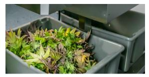
Place a tote under the front of the machine to collect the flowers and leaves and a second tote under the back of the machine to collect the chipped stalks.
