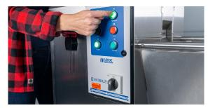
Press the FORWARD button to start the rolls and rotate the speed dial to your desired setting.
