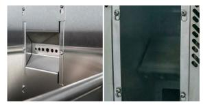
To get started, position the MBX in your work area, lock the casters and check that the front die plate and rear guard window are secured in place.
