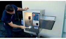
Allow the rollers and chipper to spin while the rest of the machine is sprayed with the cleaner to remove any plant debris and residue. You can use a soft brush to clean off any plant material that is more difficult to remove
