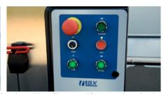
Plug the machine in, disengage the lockout and turn it on, making sure to select 'reverse direction'
