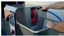
Remove the dieplate covering the rollers and rinse with water
