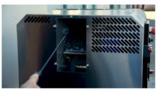
Spray the chipper, rotating it to spritz all sides with cleaner, and continue spraying the interior surfaces
