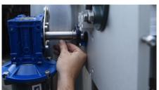
Turn the shaft of the lower flange so that it aligns with the key way on the motor gearbox. With the gearbox on about 1/2 an inch of the shaft, take the key and hold it in the key way
