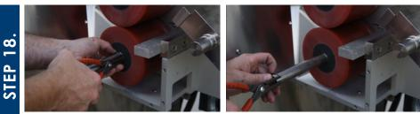
Using the circlip pliers, remove the circlip around each roller. It's advisable to wear safety glasses during this portion as the circlips can spring off and cause injury.
