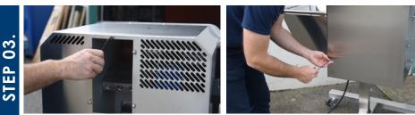
Remove the centre screw with the 3/16 allen wrench, and the 2 button-head screws at the bottom of both side panels.
