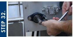
Tighten one of the bolts by hand, then pivot the other side up slightly to get that bolt started, then slide the bearing tight against the plate. Continue to thread the bolts by hand, then tighten with the socket.
