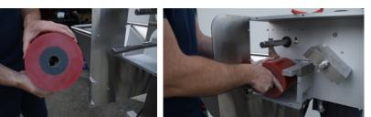
The bottom roller has a keyway. Line that up with the key and slide the roller on.
