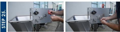
Using blue loctite, replace all seven of the screws on the side plate. Get them all started, but don't tighten until all seven are in place. You can then go back over each and snug them all down, then go back a third time to tighten them.
