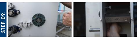
The flange should pull right off, but if it doesn't, rotate it about 45 degrees so that the holes don't line up anymore, then take 2 of the 4 bolts you removed and insert on the opposite side of the plate kitty-corner to each other.
