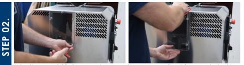
Using the same 5/32 allen wrench, remove the cover over the chipper and set aside.
