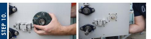
This will help push the bearing block out. Remove those bolts before moving on.
