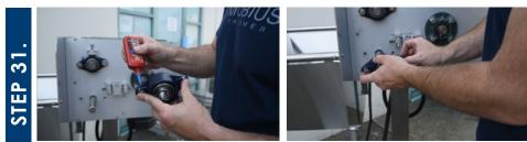
Make sure that the plastic bushings are installed in the 2 bolt lower flange bearing. Add loctite to the two bolts, then slide the bearing onto the shaft.
