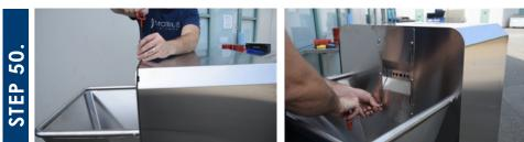
Tighten the two button heads at the top of the shroud, the two previously threaded button heads at the bottom of each side, and the 4 screws in the corners of the dieplate.
