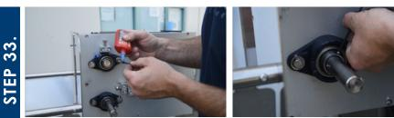
With all the flange bearings installed, you want to remove each of the 6 set screws (2 in each bearing), add a bit of blue loctite, then reinstall them using the 1/8 hex wrench. The 4-bolt flange bearing uses the 3/32 hex wrench.
