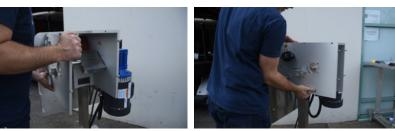
Replace the side plate making sure that all of the holes and two shafts line up properly. The top bearing will need to be moved up to line up with the shaft. Once aligned, the plate can be pushed on the rest of the way.
