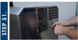
Replace the cover over the chipper and tighten each of the screws.
