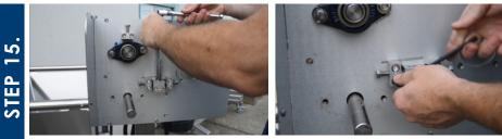
The reason for removing this portion – the adjuster bolt body – is because there is a deflector plate in behind, which will be easier to slide back in with that portion out of the way.
