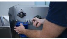
Using blue loctite, replace all seven of the screws on the side plate. Get them all started, but don't tighten until all seven are in place. You can then go back over each and snug them all down, then go back a third time to tighten them.
