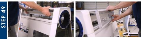
Install the brush bar by pushing it into the receptacles on either side of the lid. Both sides of the brush bar are identical so it can be installed in either orientation. Re-install the front screen
