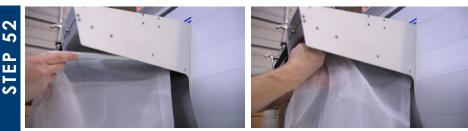
Slide the retaining ring up into the housing past the rail and allow it to fall into place. Give it a slight tug to make sure it's seated properly.
