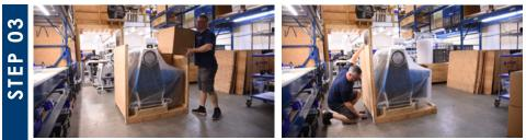
Inside the crate you'll find 2 boxes containing the hopper and chute. Remove and set them aside for later. Now, remove the remaining 3 side panels.
