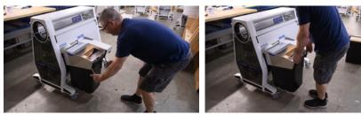
Swivel the latches towards you slightly and up so that it raises the Trim Tote and seals off the gasket, locking it in place.
