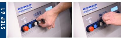
To adjust blade speed, tumbler speed and vacuum pressure, twist the dial to adjust speed and pull it out to engage the corresponding function. Turn each dial to the highest level, then dial back to achieve the trim quality you're looking for.
