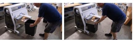
To install the Trim Tote, slide it on the rails of the separator with the warning symbol going in first.
