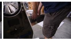
To lock the separator in place, pull the hockey stick lever up with a bit of force so that the top of the stick is flush with the top of the separator.
