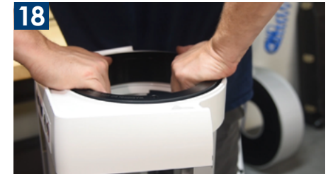
18 Just to be sure, always do a final check to make sure the tumbler retaining rings are in the fully-locked position, the tumbler is under tension, and the tumbler can rotate freely.
