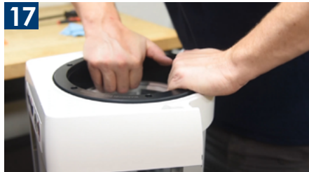
17 Grab the handles on the SpringJack and rotate the handles outward to release it from the lid.
