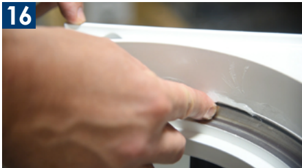
16 Now, on the SpringJack, you'll turn the air-release valve to the open position. You should see the cables of the tumbler draw tight.
