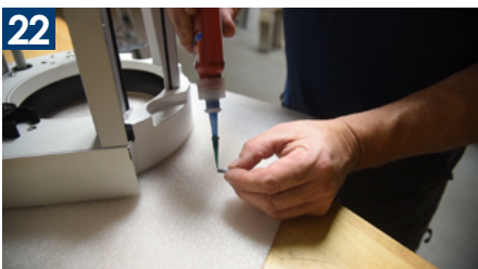
22 Install the SpringJack and pressurize
