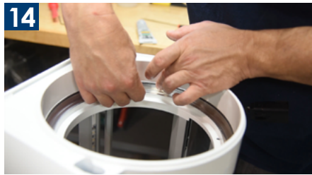
14 Now you'll lock on the outfeed side tumbler retaining ring. Our preferred method is to put your fingers just inside the tumbler, pull it towards you, and rotate the ring with your thumbs.
