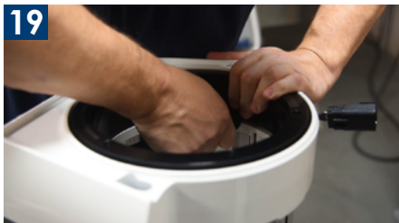
19 Replace the brush and screen and close the M108S lid.
