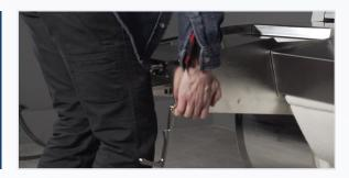
With the top side of the separator approximately parallel with the floor, begin sliding the separator into place, recognizing that the guide rail on the left side of the separator will be sliding on top of the support rail on the body of the machine.
