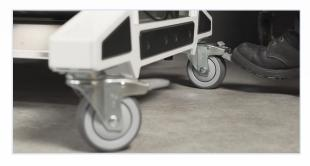
Ensure that at least two of the casters are locked so that the trimmer does not move as you are installing the separator.
