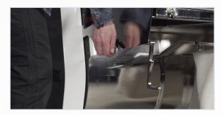
Finish the installation process by pulling up on the hockey stick to lock the separator into place.
