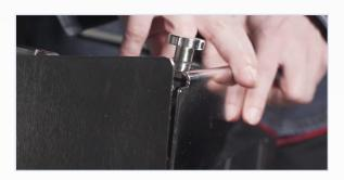
The top section is then secured into place with two tension knobs. It is vitally important that the facia and window form a tight fit with the separator body. Once assembled, the separator must be air tight so that maximum vacuum and trim quality can be achieved.
