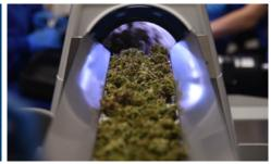
Once the tumbler is primed, turn the conveyor speed down, somewhere between 15 and 30, and maintain a consistent feed rate. Remember, load the belt with a single layer of material for consistent results.
