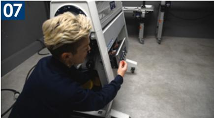
Reach in behind and push the back of the control panel to help loosen it.
