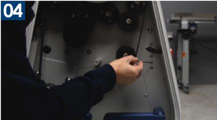
Remove the 1st and 3rd screws here as well.
