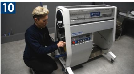
To reinstall the control panel, simply reverse the steps. Set it back inside the front body panel, and replace the first and third screw on the left side of the control panel.
