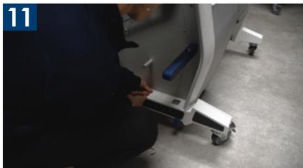
If the ebox panel was removed, replace this and install the 6 retaining screws.
