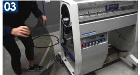
On the opposite side of the control panel, remove the clear side panel so you have access to the screws in behind.
