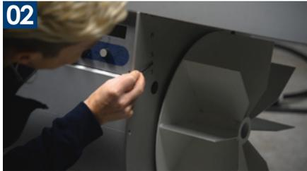
To the right of the control panel you'll see 4 screws. Remove the 1st and 3rd ones.
