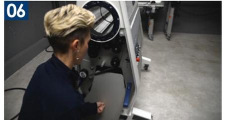
If it doesn't pop out easily, you'll need to remove the ebox panel to give the control panel a push from the back. To do this, remove the 6 small screws that hold the ebox panel in place.
