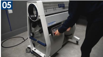
You may be able to remove the control panel easily by gently pulling on the knobs from the front.
