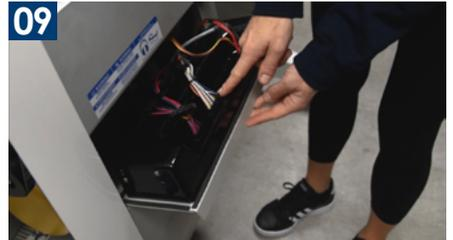
The harness in the middle connects back to the fan, blade and tumbler VFDs and the harness on the right connects back to the linear actuators for the machine tilt.
