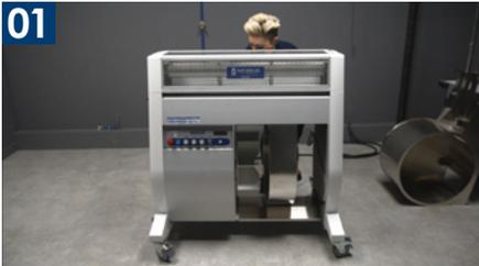
With the machine unplugged, remove the separator and fan housing from the M108S body.
