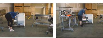
Slide the fan housing onto the 2 pegs, then install the separator,
