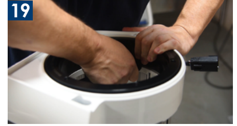
19 If your black ring gets pushed too far down on one side, use your plastic pry to remove it. Double-check there isn't any debris in the Edna and try again
