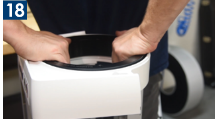
18 Begin pressing down on the black ring. Use your fingertips between the black ring and Edna to act as a buffer, preventing over-pressing in that spot.
