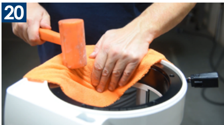
20 Once you get the O-ring gripping the bearing, you may need to use a soft deadblow mallet to seat it all the way home. Use small, even taps to finish seating the black ring.
