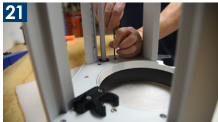
21 Let's reinstall the hex bar. Loosen the bolts and slide it back into position.
