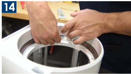
14 Press the cord into the groove, again being careful not to stretch it in the process.
