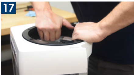
17 Set the black ring onto the O-ring, ensuring an even touch-down
