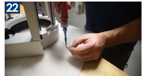
22 Remove each bolt one at a time. Apply blue Loctite to the leading threads and reinstall that bolt before removing the next bolt
