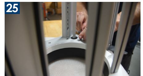
25 Tighten the bolts. This prevents excessive gear-lash. Repeat on the other end of the lid, and you're all done!
