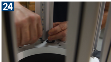
24 Push the hex bar away from the black ring that fraction of an inch that's available.
