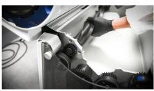
Start with the helical blades. One end has a gear, which fits to the gears on the side of the M108. Make sure the helical blades are seated properly at both sides.
